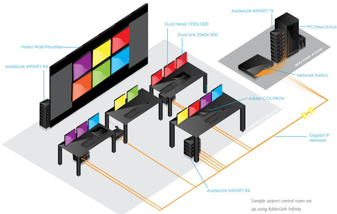
Sample airport control room set up using AdderLink Infinity
