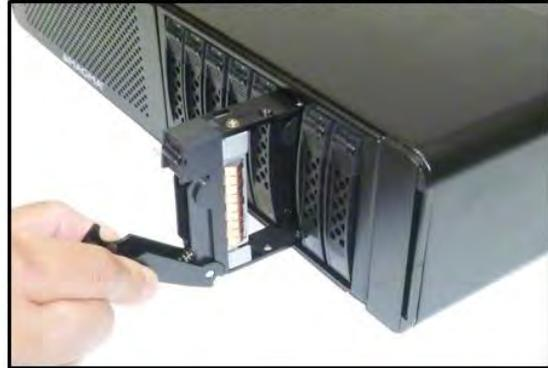
Remove the metal retainer
