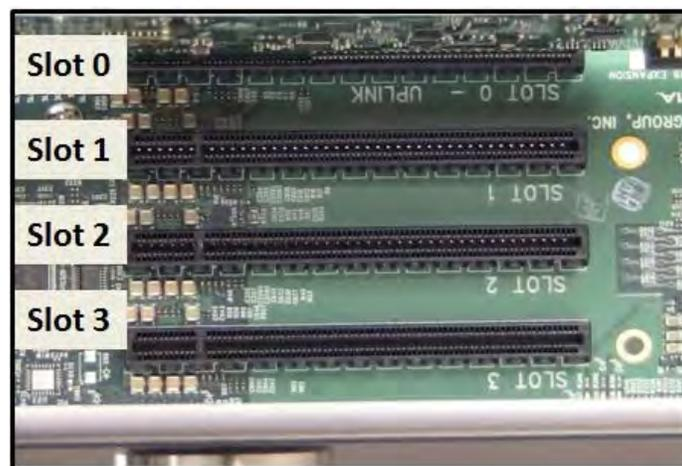
Remove slot covers and install PCIe cards.
