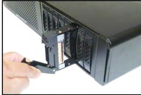
Remove the metal retainer
