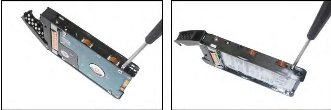
Prior to putting the drive tray back into the drive bay make sure the front mechanical latch is released. Slide the drive tray all the way in slot and then press the mechanical latch to secure.
