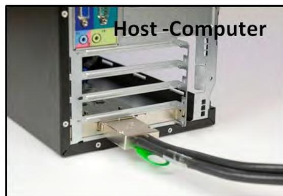
2. Connect the other end of the cable to host computer via Host Interface card.
