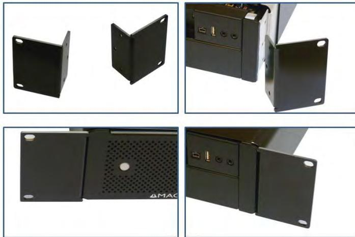
3. Mount the left and right extender rails to rear panel of the unit as shown from the pictures below.
