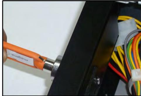
4. Push the key and rotate counter clockwise until it stops as shown from the pictures below.
