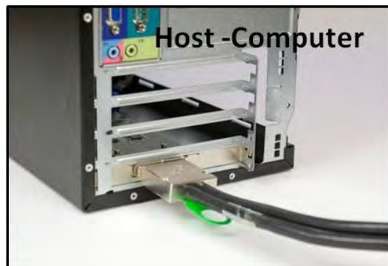
2. Connect the other end of the cable to host computer via Host Interface card.
