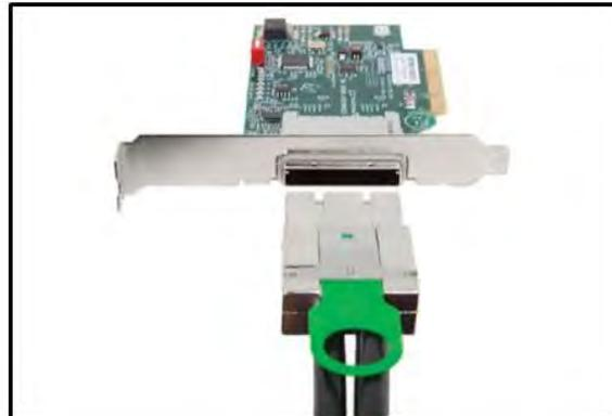
1. Connect the Ipass cable to Expansion port on the back of the unit.
