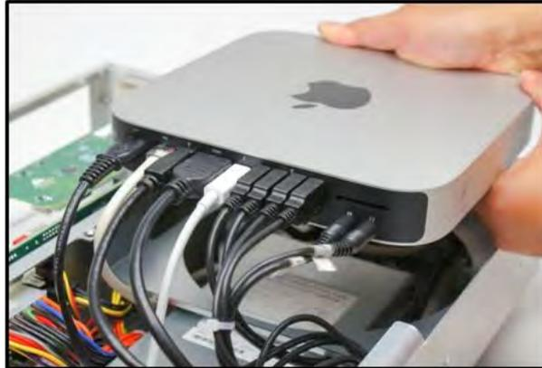
3. Place the Mac mini inside the chassis as shown from the picture below. Position the Mac mini where all cables are facing towards the front end.
