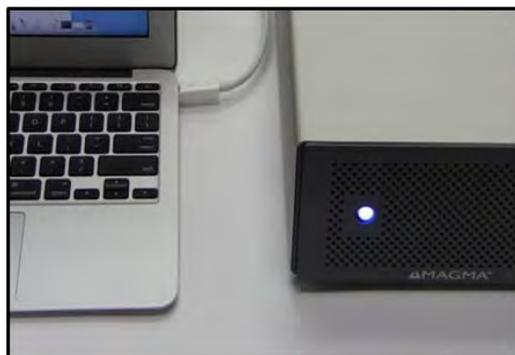
The White light on the front of Roben-3 is not an ON (On-off push button), it simply indicates whether the chassis is on or off. If either end of the Thunderbolt cable is disconnected, Roben-3 will automatically turn off.
